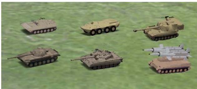
Fig. 2. The image shows the six CAD models with textures for visual wavelengths that is used in the simulations. From the upper left: BMP 1, BTR 80, M109A6, T72, T80, SA4 launch vehicle.
