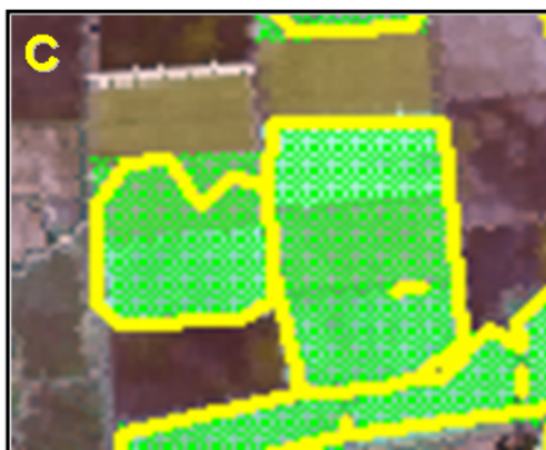
Figure 5. Extraction of Land Cover (Agricultural Areas) Using ALPHATECH's Neural Fusion Software. Images A and B show the raster level extraction performed by two different analysts. Figure C shows the vectorized result (in yellow), compared to the manual extraction manual extraction (in green).
