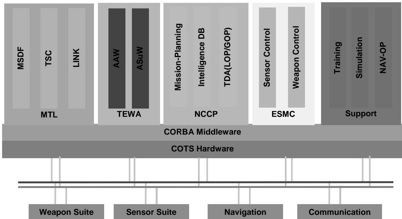
Figure 2: Modular Advanced Naval Combat System Software Architecture
