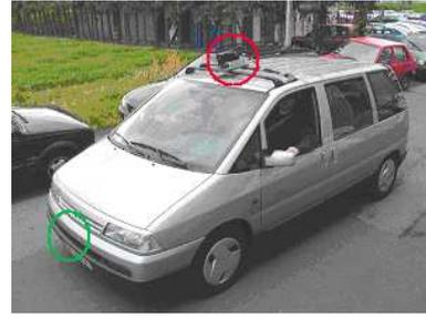
Fig. 4: VELAC equipped with IR and Radar
