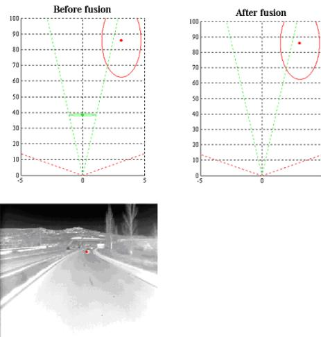
Fig. 14: Radar detection not confirmed by infrared
