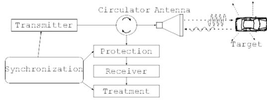
Fig. 5: Structure of the PAROTO Radar with one antenna
