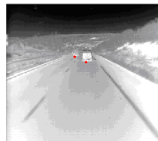
Fig. 11: Data Fusion on simple situation (red = Infrared, green = Radar, blue = dual-mode)
