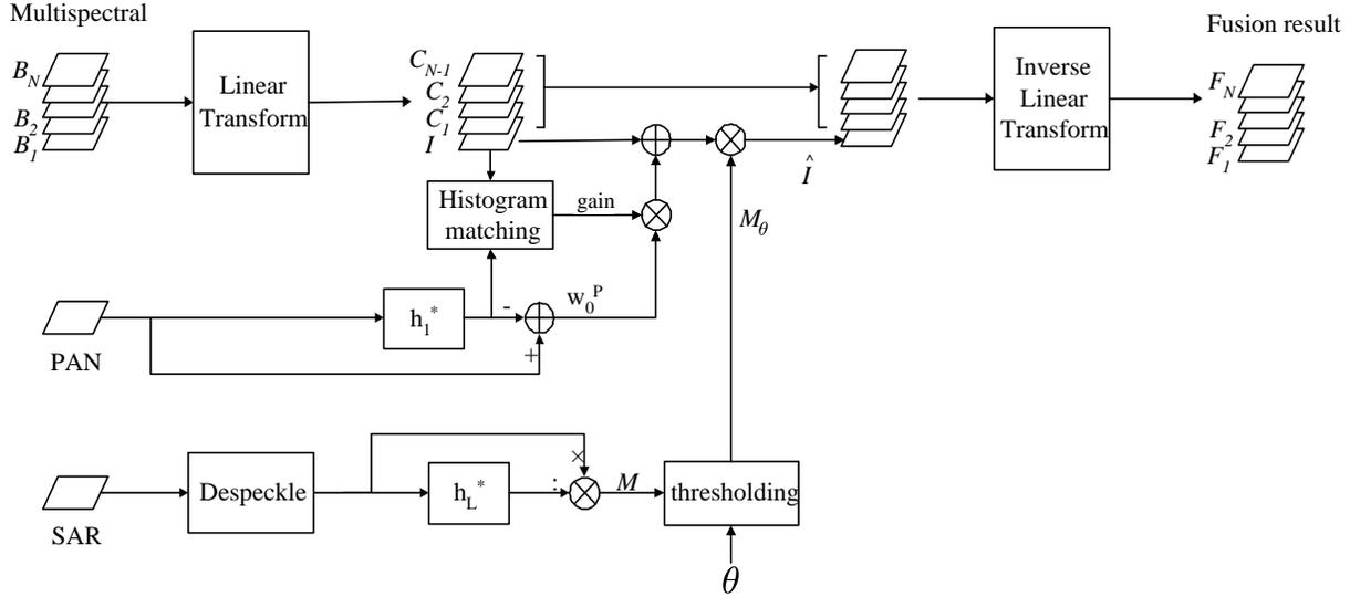
Fig. 1: Flowchart of the procedure for fusion of a low-resolution  $N$ -band MS image with a high-resolution Pan image and a high-resolution SAR image. The MS bands are preliminarily resampled at the finer scale of the fusion product by means of bicubic interpolation.
