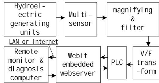
Fig. 2. Principle frame chart of network on-line detection.
