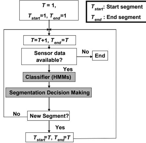
Figure 6. Integrated HMM classification and segmentation process.
