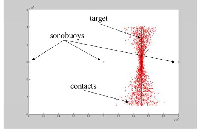
Fig. 2. Visualization of geometry for benchmark problem, with one realization of sonar contacts overlaid. Target motion is in the  $-y$  direction. The total scale is  $20\text{km}$  in the  $x$ -dimension, and  $120\text{km}$  in the  $y$ -dimension.
