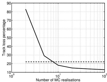
Fig. 3: Track loss percentage of bootstrap filter with proposed gating scheme (solid) plotted against number of MC realisations used in gate volume estimation. Results are shown for  $n = 200$  particles. The performances of the PDA-EKF and bootstrap filter with Gaussian gating scheme are indicated by a dotted line and dashed line, respectively.
