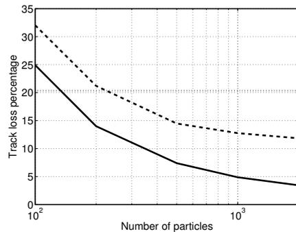
Fig. 5: Track loss percentage of bootstrap filter with proposed gating scheme (solid) and Gaussian gating scheme (dashed) plotted against number of particles.  $s = 50$  realizations are used to estimate the gate volume. The performance of the PDA-EKF is indicated by a dotted line.
