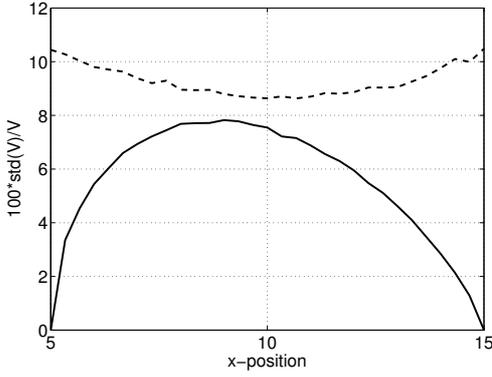
Fig. 1: Normalised standard deviation of the naive estimator (dashed) and the overlap estimator (solid) plotted against the  $x$ -position of the second gate. The first gate is at  $x = 5$ . Both gates have radius 5.
