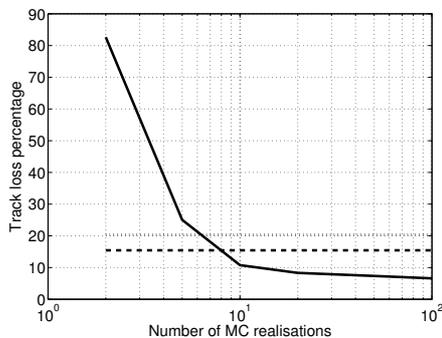
Fig. 4: Track loss percentage of bootstrap filter with proposed gating scheme plotted against number of MC realisations used in gate volume estimation. Results are shown for  $n = 500$  particles. The performances of the PDA-EKF and bootstrap filter with Gaussian gating scheme are indicated by a dotted line and dashed line, respectively.
