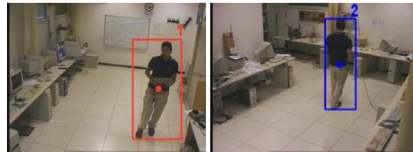
Figure 6. Sample processed frames indicating Blobs (i.e.: moving objects) and their centers of mass from two Fields of View.
