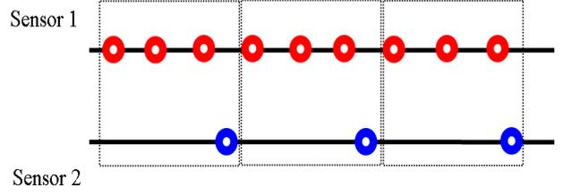
Fig. 2: Asynchronous Sensors with Different Rates
