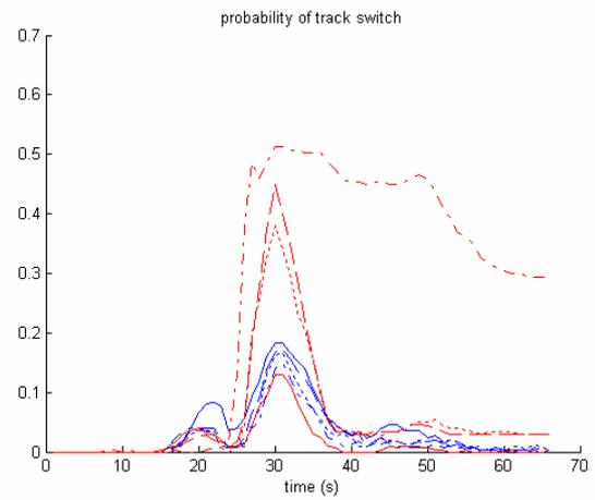
Fig. 7. Scenario 1. Track switch probability for target 1
